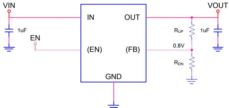
Note1: Only the SOT23-5/TDFN-4 package has an EN pin.
