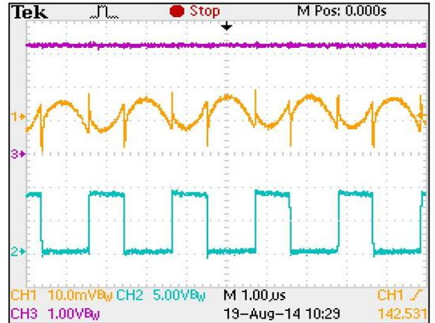
$V_{IN}=9V, V_{OUT}=3.3V, I_{OUT}=2.0A$
