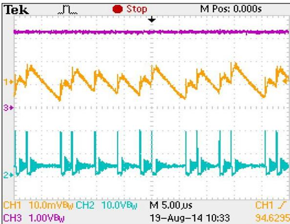
$V_{IN}=12V, V_{OUT}=3.3V, I_{OUT}=50mA$
