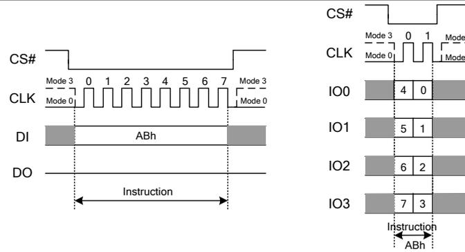
Figure 7.28 Release Power-down Instruction(SPI and QPI Mode)
