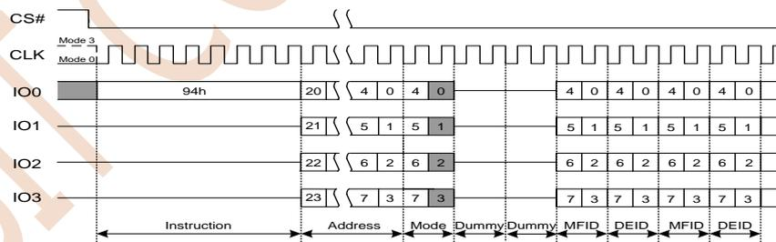
Figure 7.37 Read Manufacturer/Device ID Quad I/O Instruction
