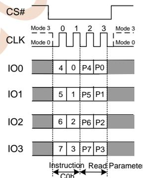
Figure 7.39 Set Read Parameters Instruction (QPI Mode only)
