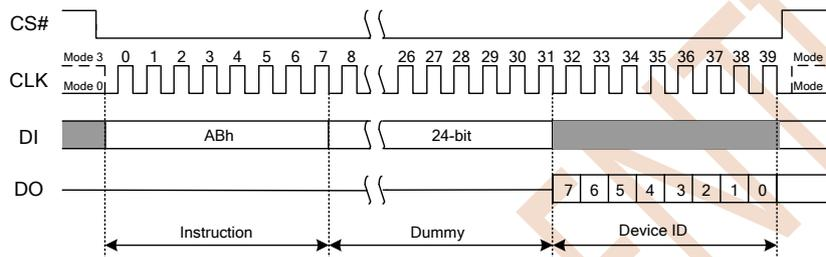
Figure 7.29a Release Power-down / Device ID(SPI Mode)
