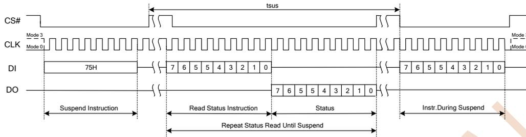
Figure 7.11a Erase / Program Suspend Instruction(SPI Mode)
