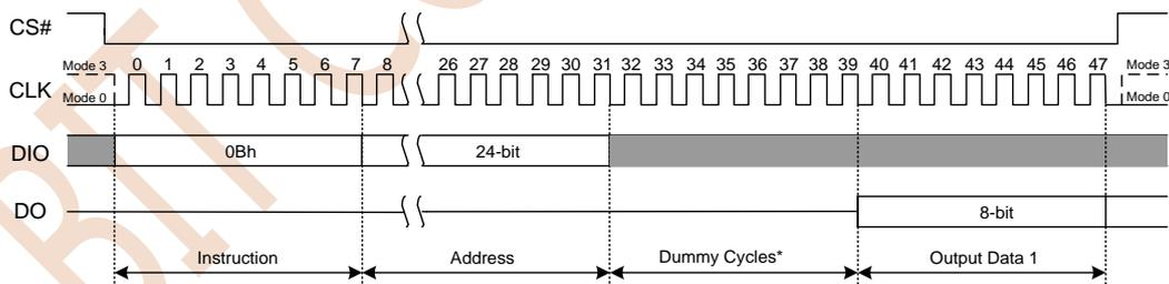
\* The Dummy Cycles is set by SR3[3:0], the default is 8 dummy, see details in Table 6.5
