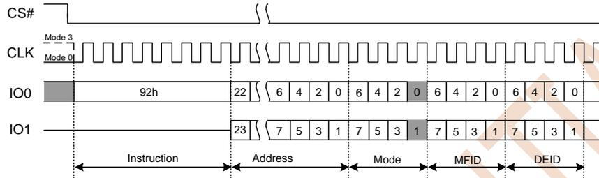
Figure 7.36 Read Manufacturer/Device ID Dual I/O Instruction
