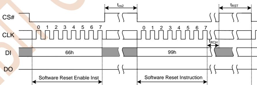
Figure 8.7 Software Reset Input Timing
