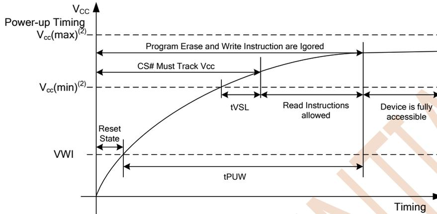
Figure 8.1 Power-up Timing
